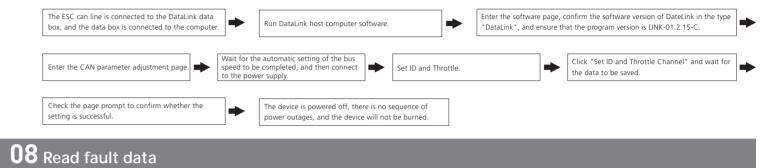
The ESC has its own fault storage function, which can store power-on times, flight time, and fault times information, which is convenient for flight fault analysis. This function needs to use DataLink data box, serial port assistant, and DataLink host computer software.
