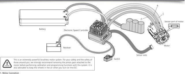
Sensored motor connection MUST connect A from the ESC to A on the motor, B to B, and C to C, with the sensor wire connected any variation of the motor to ESC connections may cause damage. Note: If the motor direction is reversed, change the parameter item "Motor Rotation" to achieve the correct setting.
