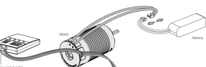
This system supports the use of LED and LCD G2/Pro program box for parameter settings. Below is an example of the setting method using the LED program box, the connection method for the LCD G2/Pro program box is
