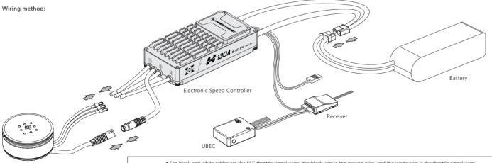
• The black and white cables are the ESC throttle signal wires, the black wire is the ground wire, and the white wire is the throttle signal wire
