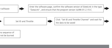
DataLink data box firmware version requirements: LINK-01.2.15-C or later; serial port assistant requirements: USB to TTL protocol; DataLink host computer software requirements: fault storage
