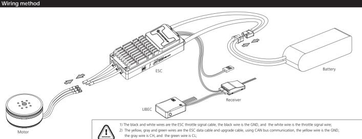
3) The CAN cable is also a digital throttle cable and can be used in parallel
